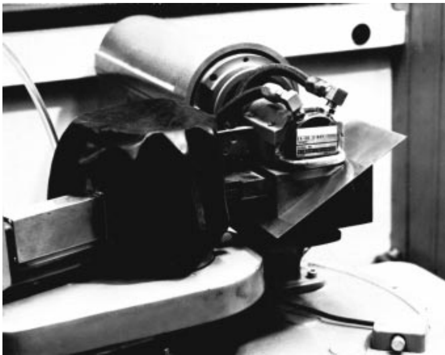
FIG. 1 Special Sample Holder for X-Ray Beam Exposure
