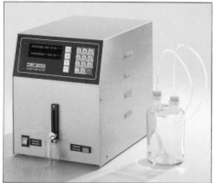
FIG. A1.2 SC 819 Automatic Cloud Point
