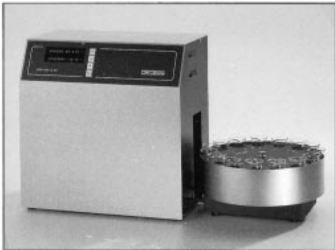
FIG. A1.1 SC 815 Automatic Cloud Point
