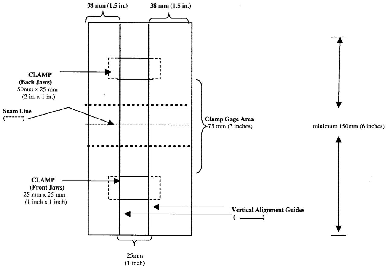
**FIG. 1 Specimen Placement in Clamps
