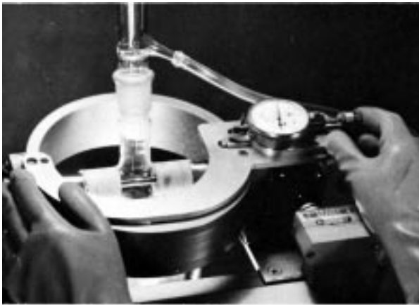
FIG. 2 Spring-Loaded Stressing Frame (7)
