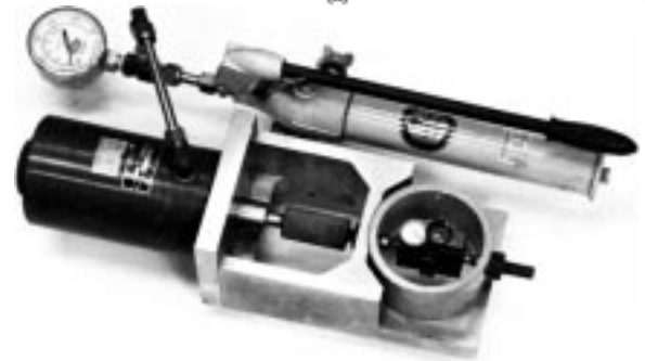
FIG. 3 Sustained Load Devices Using Ring Frames (8)
