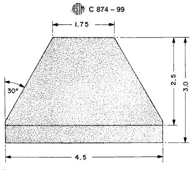
NOTE 1—Dimensions are in inches. NOTE 2—Six cuts are needed for complete lining.
