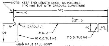
NOTE: ALL DIMENSIONS IN MILLIMETERS TOLERANCES: ± 0.5 mm
