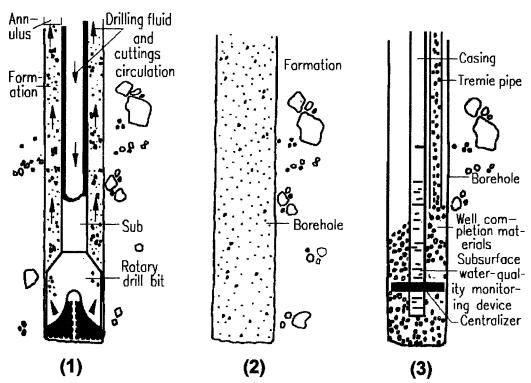
FIG. 1 Sketch Showing Basic Three-Step Procedure for Installation of Subsurface Water-Quality Monitoring Device Using Direct-Rotary
