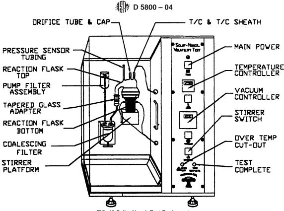
FIG. 13 Selby-Noack Test Equipment
