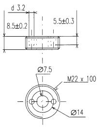
FIG. 12 Extraction Tube Nut (Stainless Steel) (Detail 5 of Fig. 7)
