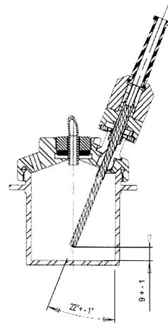
FIG. 10 Specimen Temperature Probe Positioning
