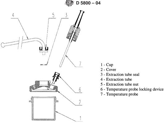
FIG. 7 Crucible with Temperature Probe
