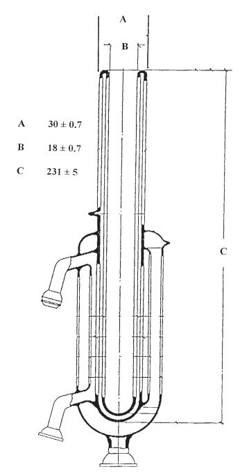
Note 1—All wall thicknesses are  $2\pm0.1$  mm. Note 2—All dimensions are in millimetres. FIG. A1.1 Test Chamber
