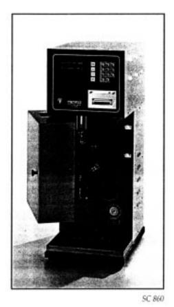
FIG. A1.4 Automated Freezing Point Apparatus
