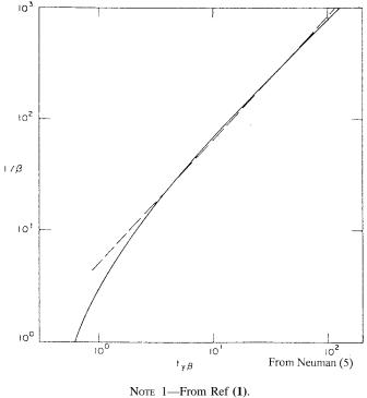
FIG. 5 Values of  $1/\beta$  Versus  $t_{y\beta}$  for Fully Penetrating Wells
