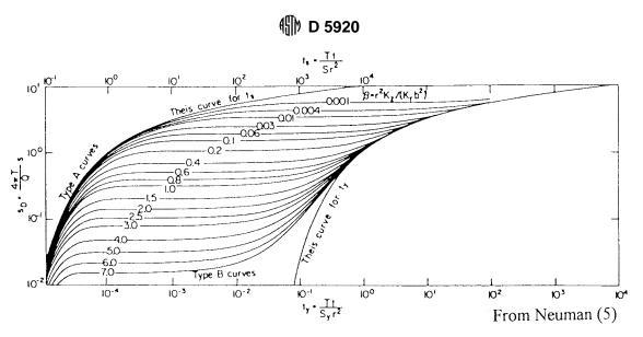
NOTE 1—From Ref (5). FIG. 3 Type Curves for Fully Penetrating Wells
