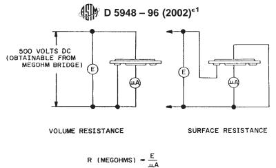
FIG. 4 Circuits for Measuring Low Values of Volume and Surface Resistance
