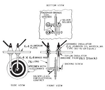
Note 1—All dimensions in millimetres. Note 2—Material — brass except as indicated. Note 3—Silver plate all metallic parts except plate. FIG. 2 Specimen Holders Electrodes Test Samples and Humidity Chamber Cover—Volume and Surface Resistance Test
