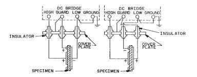
VOLUME RESISTANCE SURFACE RESISTANCE FIG. 3 Arrangements for Volume Resistance and Surface Resistance Test
