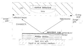
FIG. A1.1 Schematic of Test Chamber
