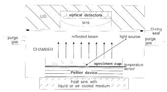
FIG. A1.2 Detection of Crystal Formation
