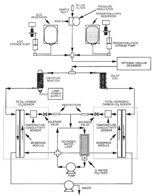
FIG. 1 Schematic Diagram of TOC Analyzer System
