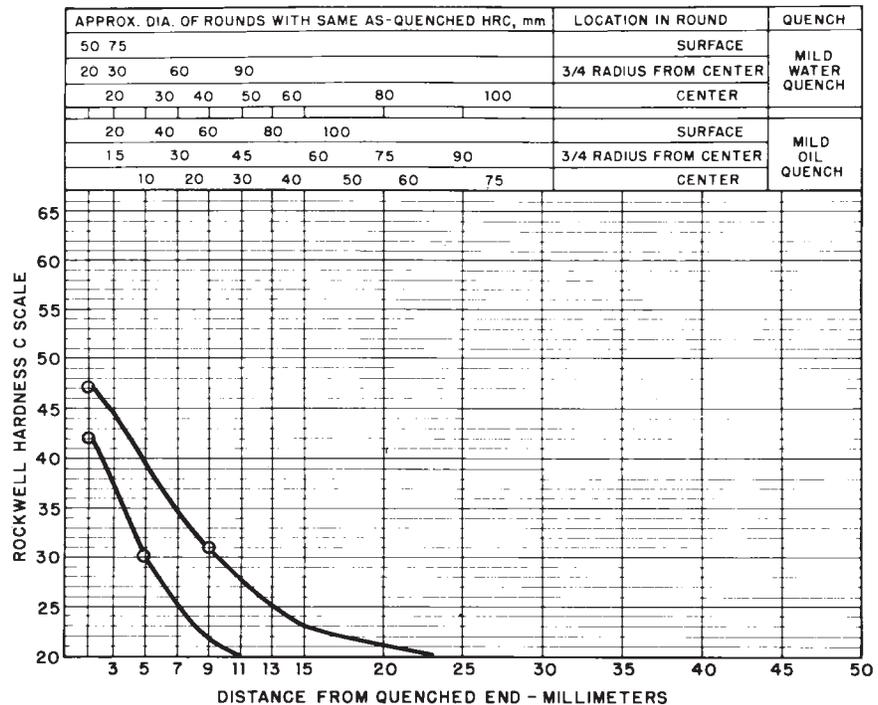
FIG. 13 Limits for Hardenability Band 4620 RH
