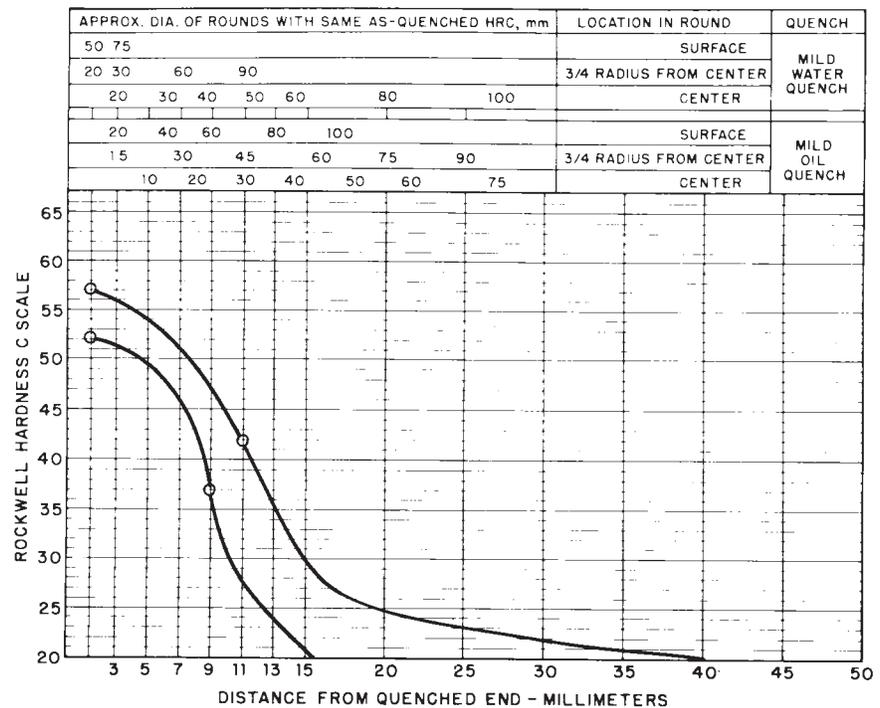
FIG. 3 Limits for Hardenability Band 15B35 RH
