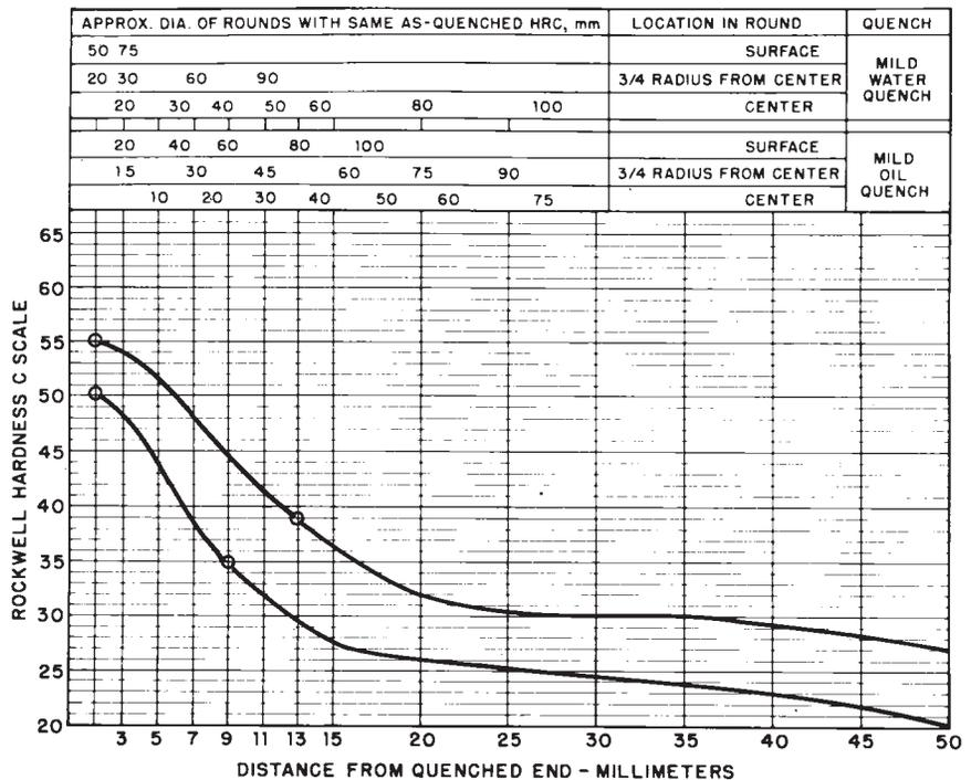
FIG. 8 Limits for Hardenability Band 4130 RH
