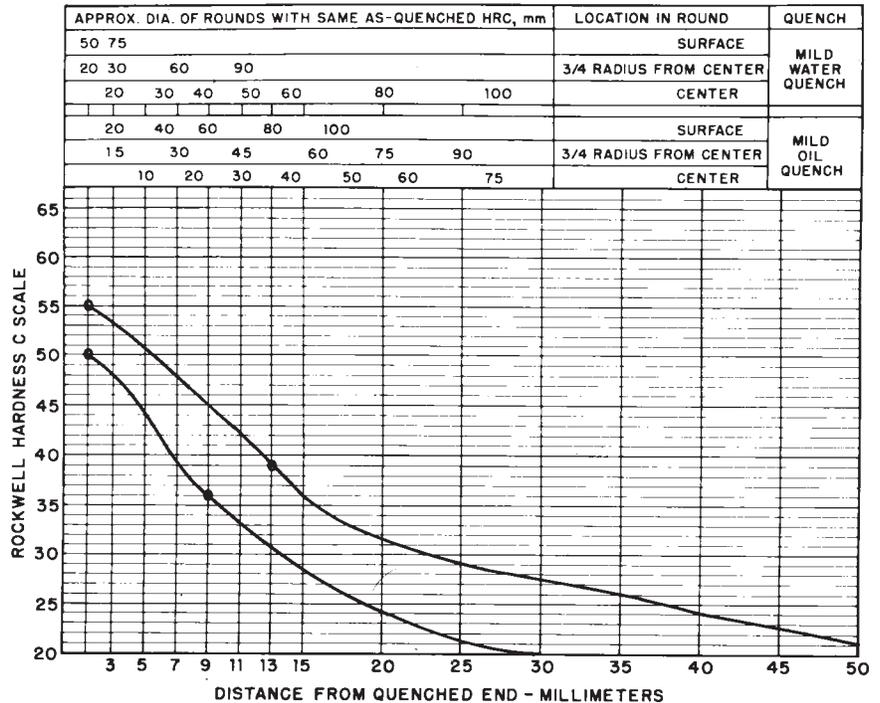
FIG. 16 Limits for Hardenability Band 5130 RH
