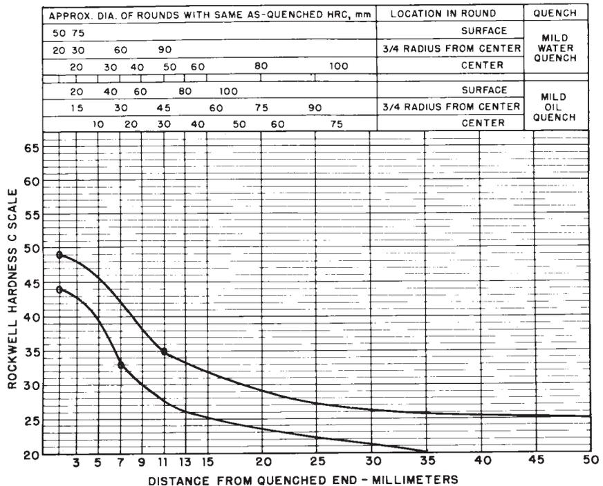
FIG. 22 Limits for Hardenability Band 8822 RH
