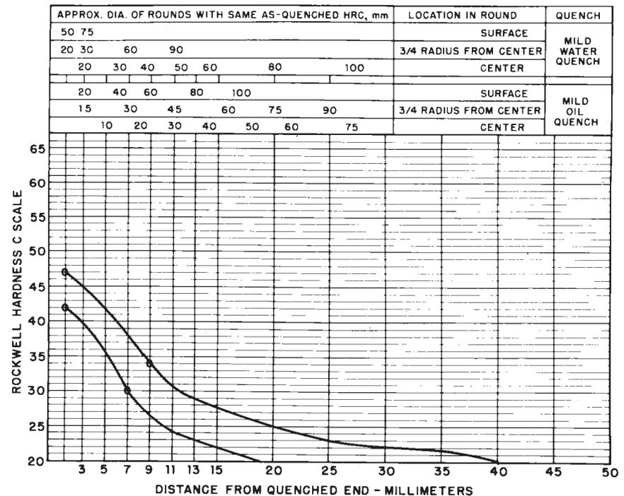
FIG. 21 Limits for Hardenability Band 8720 RH
