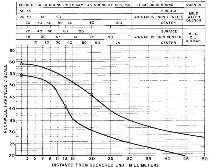
FIG. 15 Limits for Hardenability Band 50B40 RH
