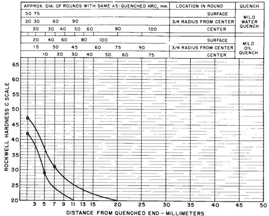
FIG. 6 Limits for Hardenability Band 4118 RH
