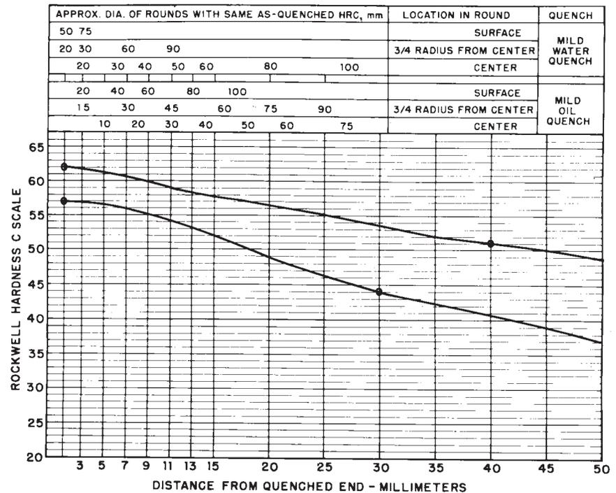
FIG. 11 Limits for Hardenability Band 4161 RH
