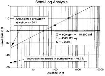
FIG. 3 Extrapolation of Straight Line on Semilog Graph
