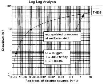
FIG. 6 Extrapolated Drawdown for Partially Penetrating Well
