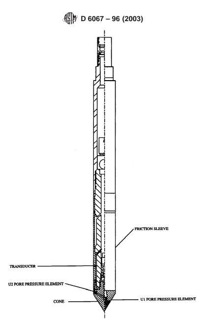
FIG. 1 Electronic Cone Penetrometer
