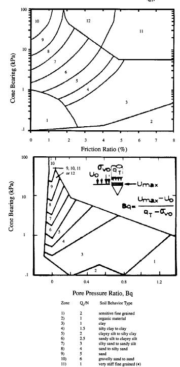
(•) over consolidated or cemented FIG. 2 Simplified Soil Classification Chart for Standard Electric
