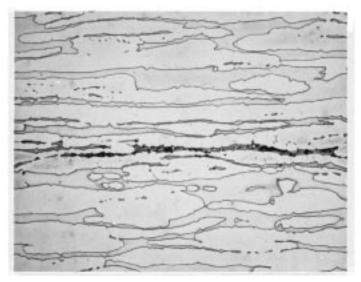
FIG. 7 S31803: Longitudinal Section (500× Magnification Before Reproduction)
