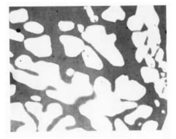
FIG. 4 (a) J92205: Possibly Affected Structure-Statically Cast  $(400 \times \text{Magnification})$
