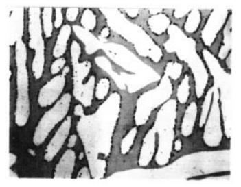
FIG. 6 J92205: Affected Structure (400× Magnification)
