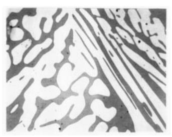
FIG. 2 (b) J92205: Unaffected Structure-Centrifugally Cast (400× Magnification) (continued)
