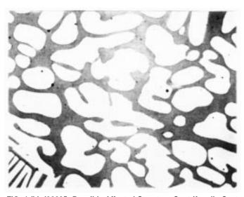
FIG. 4 (b) J92205: Possibly Affected Structure-Centrifugally Cast (400 $\times$  Magnification) (continued)
