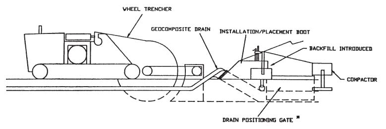
Note 1—Drain positioning gate should be located and adjusted to position, and hold the geocomposite drain against the trench wall, to prevent possible "J"ing or "C"ing of the drain during backfilling and compaction.
