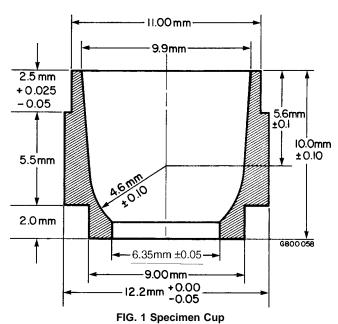
filled with benzoic acid. Remove any crystals from the exterior of the cup.
