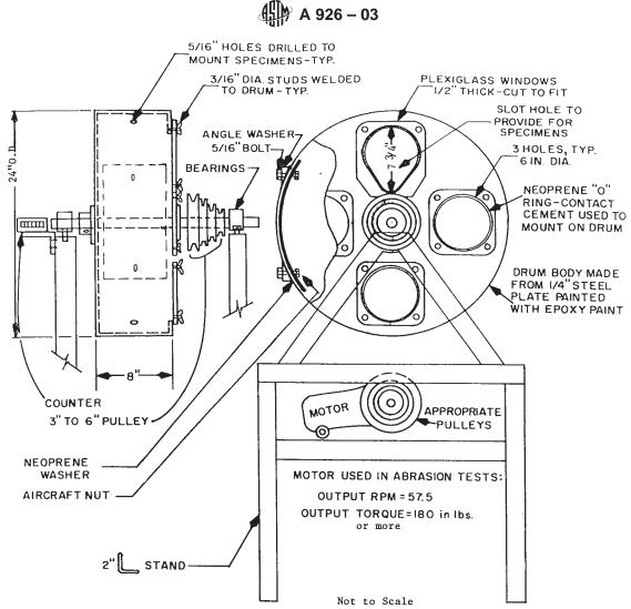
FIG. 1 Bed Load Abrasion Testing Machine
