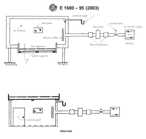
Alternate preferred if dynamic test will be performed on same specimen.
