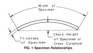
NOTE 3—The highest point will normally be at or near the center of the specimen.
