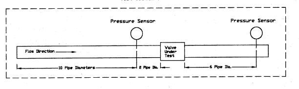
Test Section Detail
