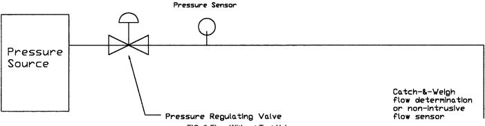
FIG. 3 Flow Without Test Valve
