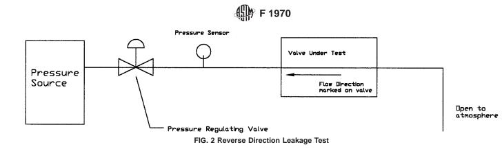
connection equal to the 1.5 times the nominal pressure of the valve and begin the timer.
