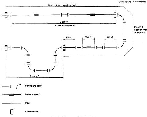
FIG. 4 Thermal Cycling Test
