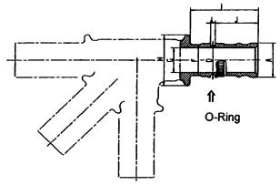
FIG. 2 Compression Fittings and O-Rings for Multilayer Pipe
