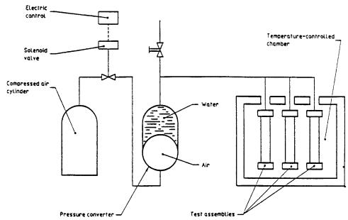
FIG. 5 Water Hammer Test
