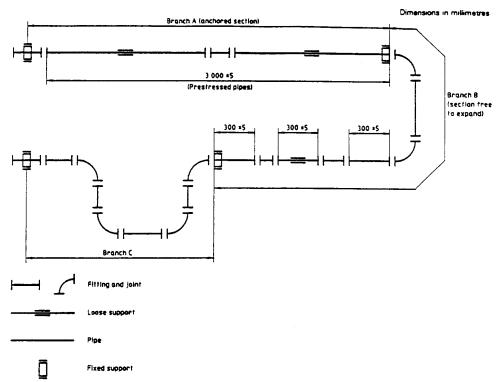
FIG. 4 Thermal Cycling Test
