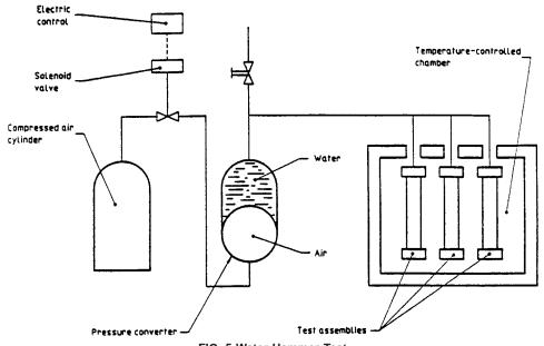
FIG. 5 Water Hammer Test
