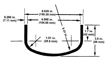
NOTE 1—Caps furnished to ANSI standards unless otherwise specified. Welding caps are formed from steel plate and are ellipsoidal in shape. The minor axis being equal to one half the major axis radii "R" and "r" closely approximate the actual semi-ellipsoidal shape. All dimensions in inches and are in accordance with ANSI B16.9.
