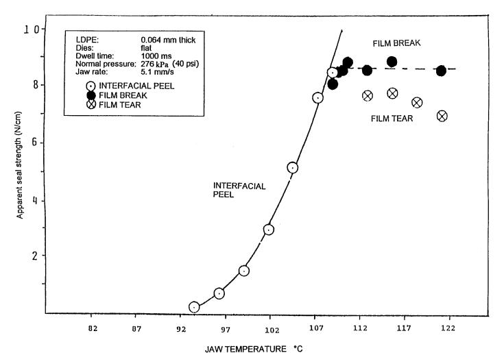
FIG. 1 Failure Modes of Seals made with LDPE Film
