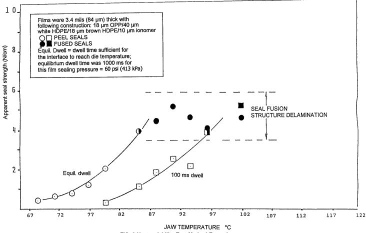
FIG. 2 Heatsealability Test Method Example
