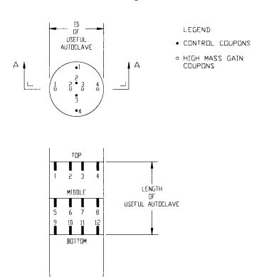
FIG. 1 Control Coupon and High Mass Gain Coupon Positioning for Establishing Mass Gain Mean and Standard Deviation
