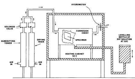
FIG. 1 Main Parts of the Cyclic Humidity Corrosion Exposure Apparatus (Schematic)
