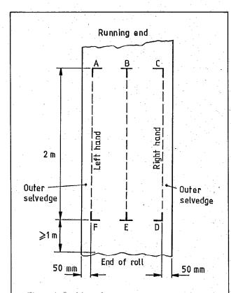
Figure 1. Position of gauge marks on the surface of the coated fabric for determination of dimensional changes on mechanical relaxation at zero tension
