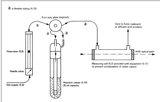
$\label{eq:Figure 2-Example of apparatus for the determination of mercury by flameless atomic absorption spectrometry$
