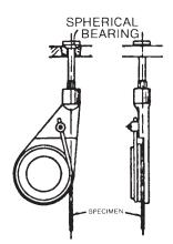
FIG. 5 Snubbing Device for Testing Wire
