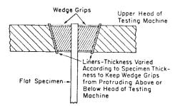
FIG. 1 Wedge Grips with Liners for Flat Specimens
