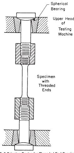
FIG. 2 Gripping Device for Threaded-End Specimens
