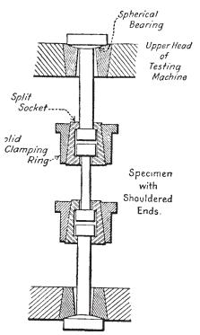
FIG. 3 Gripping Device for Shouldered-End Specimens
