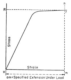
FIG. 17 Stress-Strain Diagram for Determination of Yield Strength by the Extension-Under-Load Method
