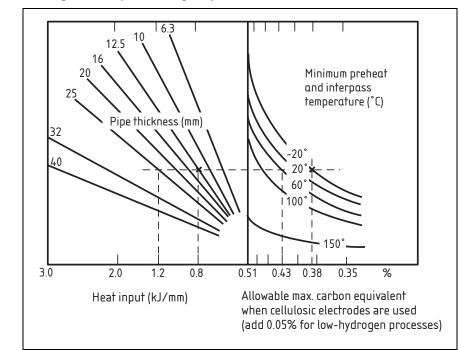
Figure E.1 Nomogram for preheating requirements
