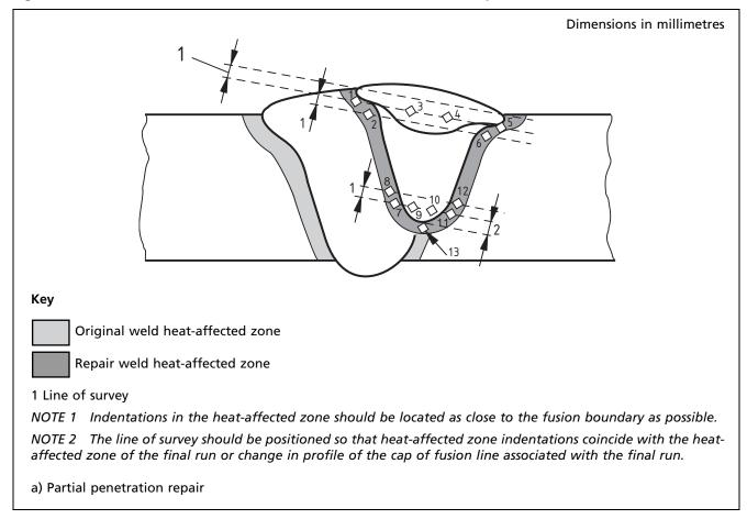
Figure 5 Recommended locations for hardness indentations for repair test welds
