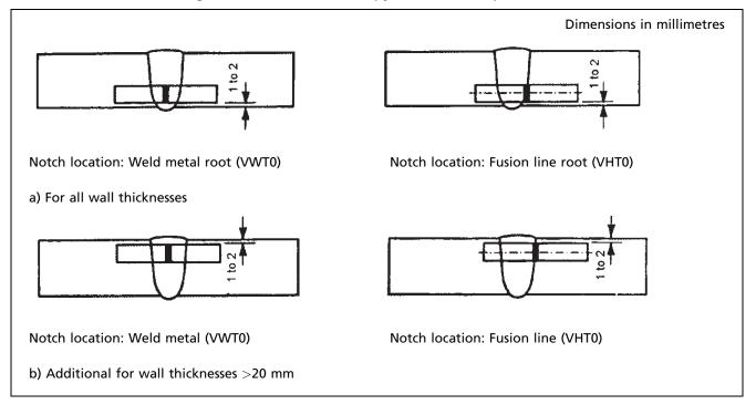
Figure 3 Position of Charpy V-notch test specimens
