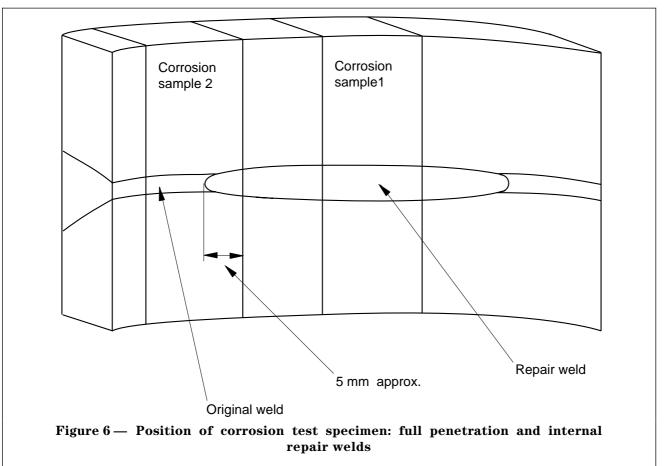
If the weight loss is >5 g/m<sup>2</sup>, the specimen shall be considered to have failed the test, unless pitting is positively identified only on areas outside of the test face.
