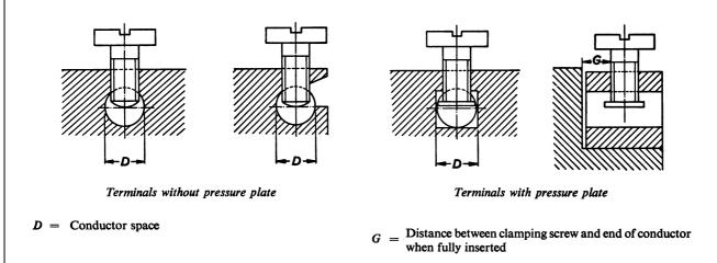
NOTE The part of the terminal containing the threaded hole and the part of the terminal against which the conductor is clamped by the screw may be two separate parts, as in the case of terminals provided with a stirrup. The shape of the conductor space may differ from those shown, provided a circle with a diameter equal to the minimum value specified for D can be inscribed.
