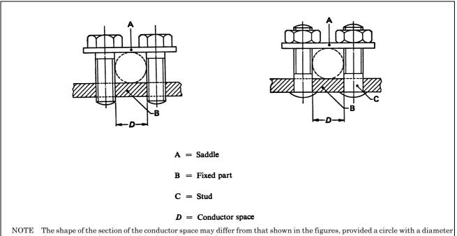
NOTE The shape of the section of the conductor space may differ from that shown in the figures, provided a circle with a diameter equal to the minimum value specified for D can be inscribed.
