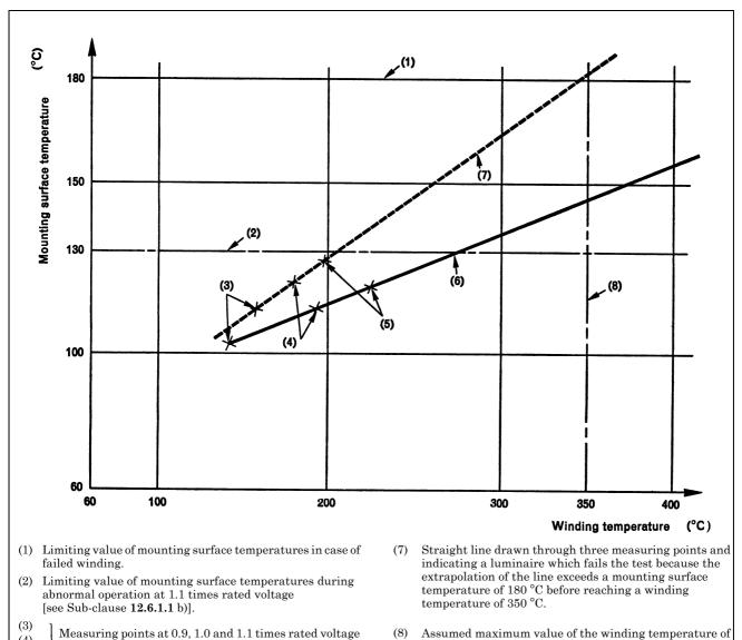
(8) Assumed maximum value of the winding temperature of a failed winding.
