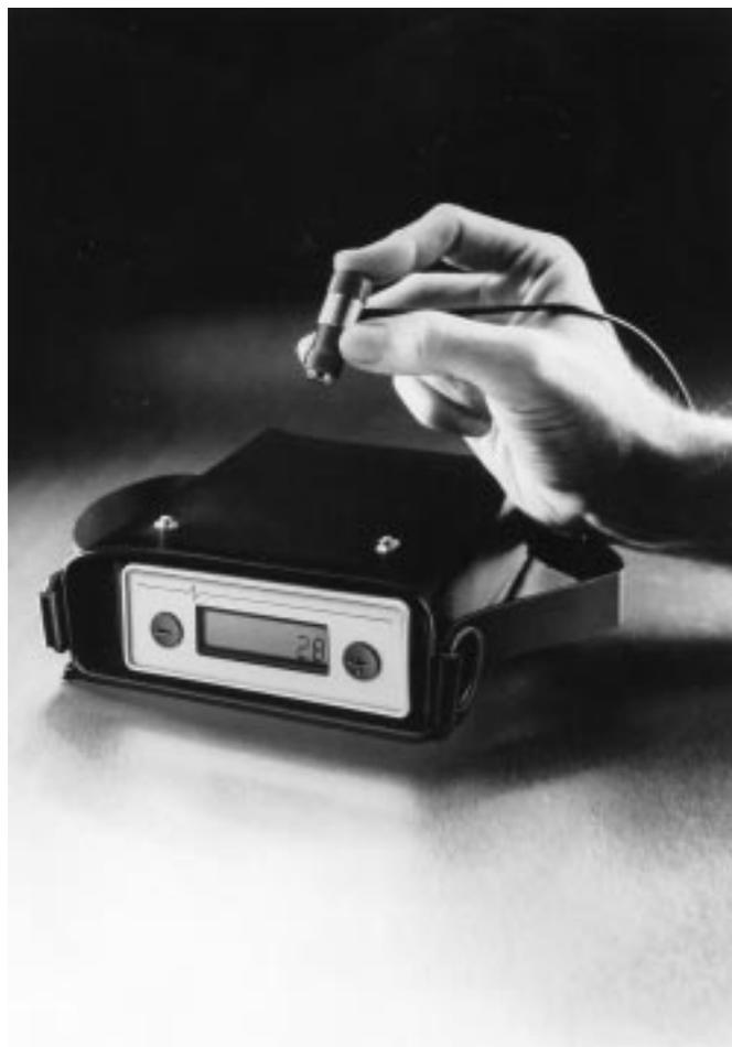
**FIG. 1 Ultrasonic Thickness Gage**
