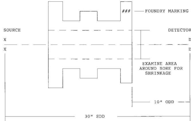
NOTE 1—Indicate scan plan details, including each required view, location of required IQIs and markers, sequence of required views, and direction and maximum speed of manipulation. Where it is impractical to place the IQI on the casting, indicate the selection and location of the appropriate mounting block and IQI.
