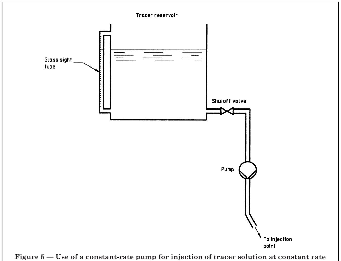
Figure 5 — Use of a constant-rate pump for injection of tracer solution at constant rate
