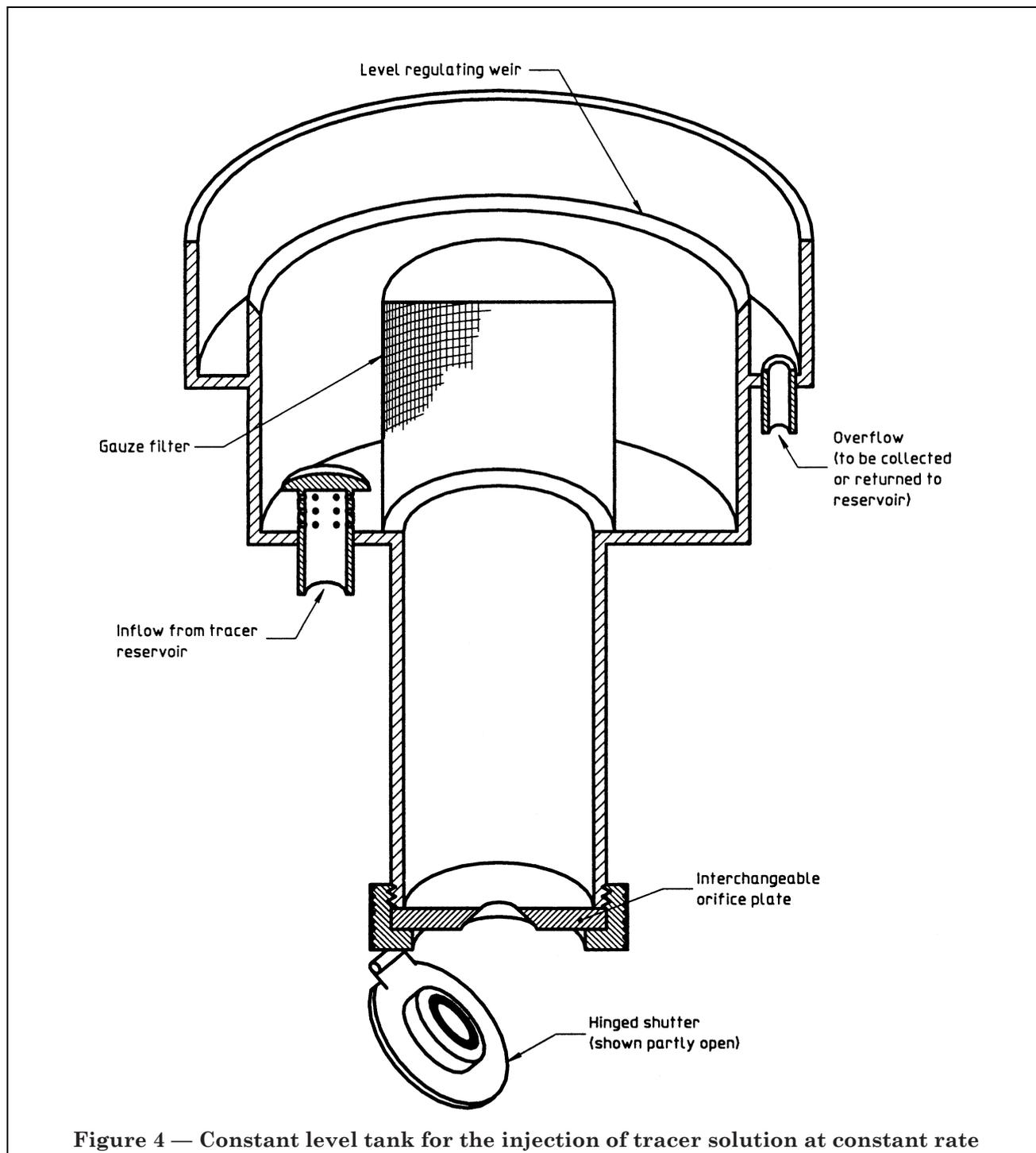
Figure 4 — Constant level tank for the injection of tracer solution at constant rate
