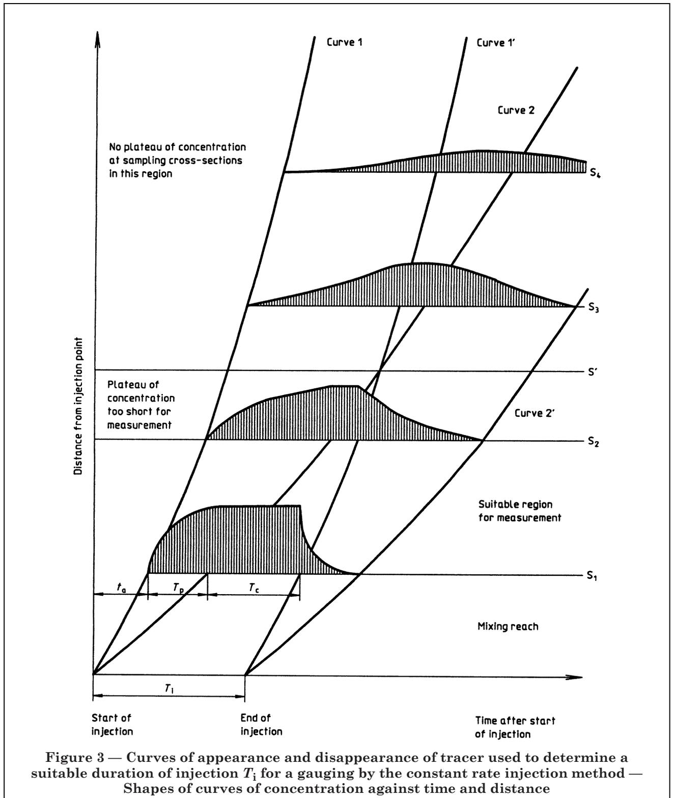
Figure 3 — Curves of appearance and disappearance of tracer used to determine a suitable duration of injection  $T_i$  for a gauging by the constant rate injection method — Shapes of curves of concentration against time and distance
