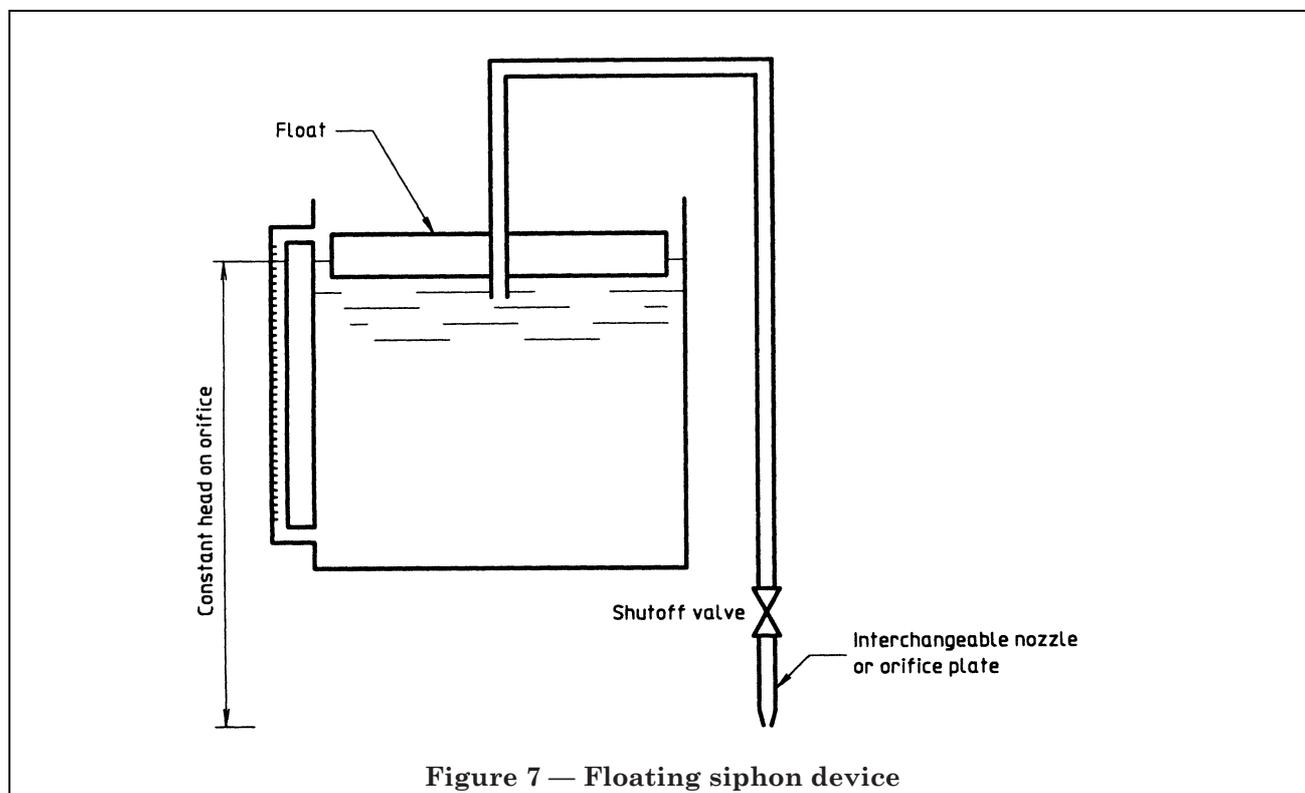
Figure 7 — Floating siphon device
