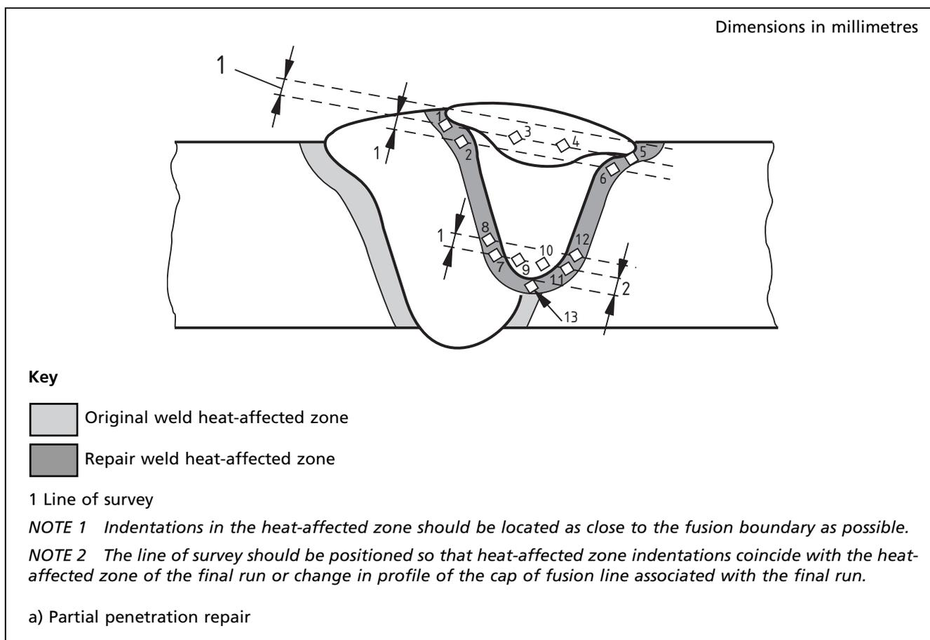
Figure 5 Recommended locations for hardness indentations for repair welds (continued)
