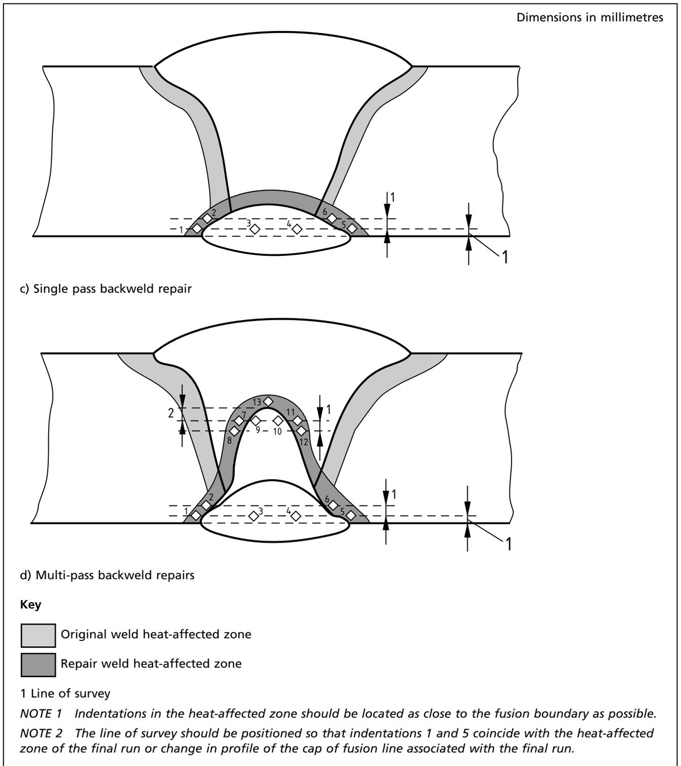
Figure 6 Positioning of Charpy V-notch impact specimens for procedure approval of partial penetration repair welds
