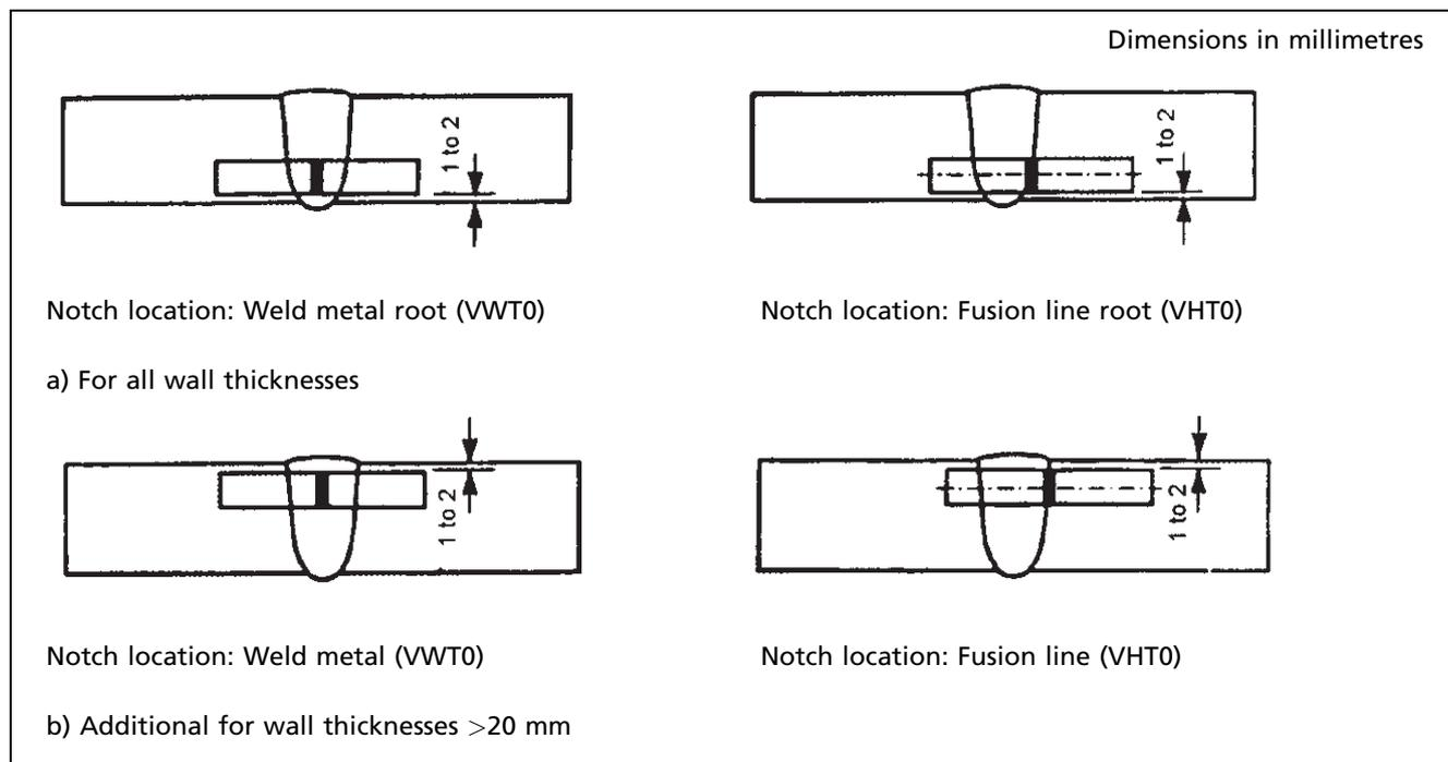
Impact test specimens shall be taken from each of the locations in Figure 1. For vertical-down welding, specimens shall be taken from 12 o'clock and 6 o'clock positions and for vertical-up welding, specimens shall be taken from 12 o'clock and 3 o'clock positions.
