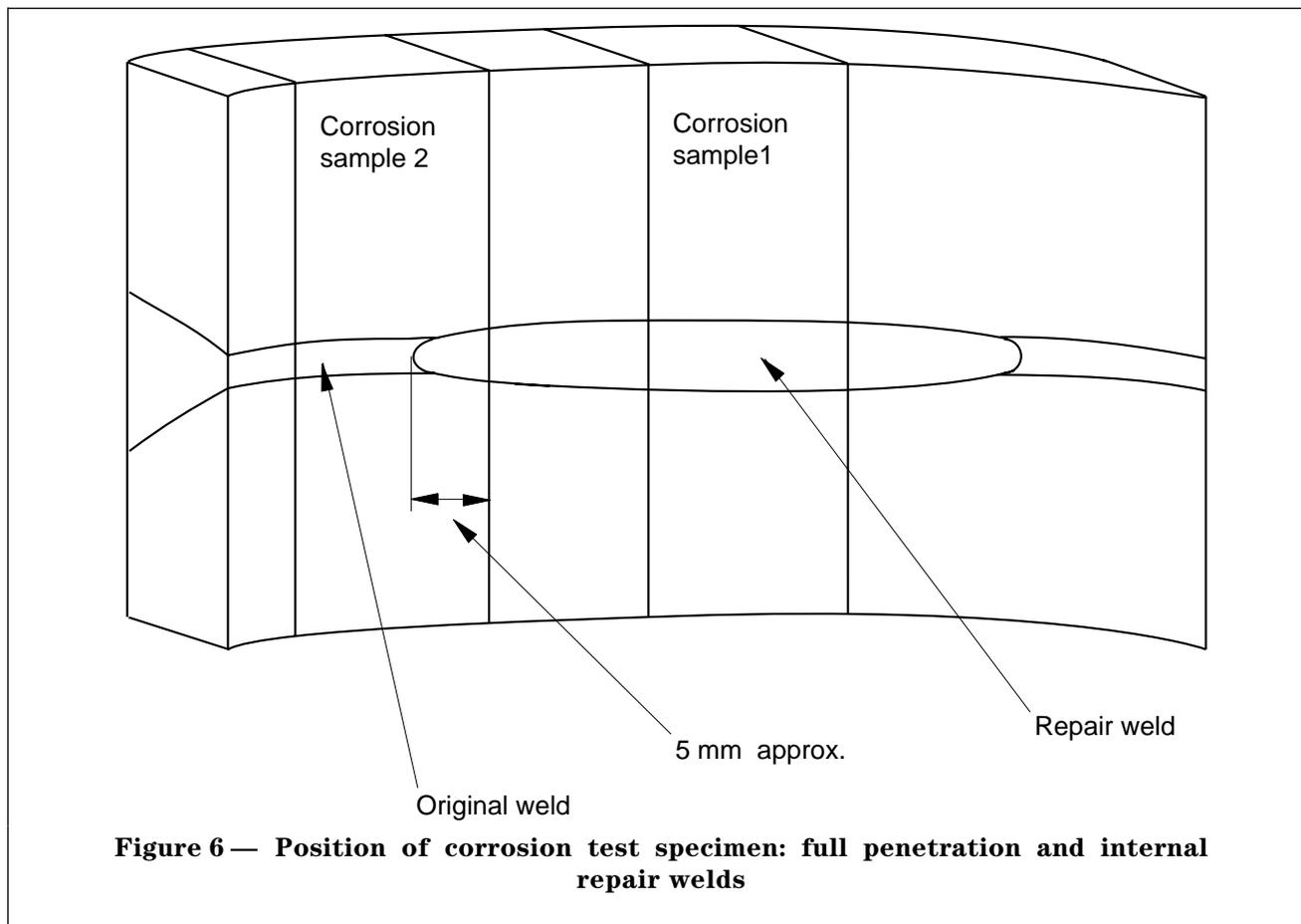
**Figure 6 — Position of corrosion test specimen: full penetration and internal repair welds**
