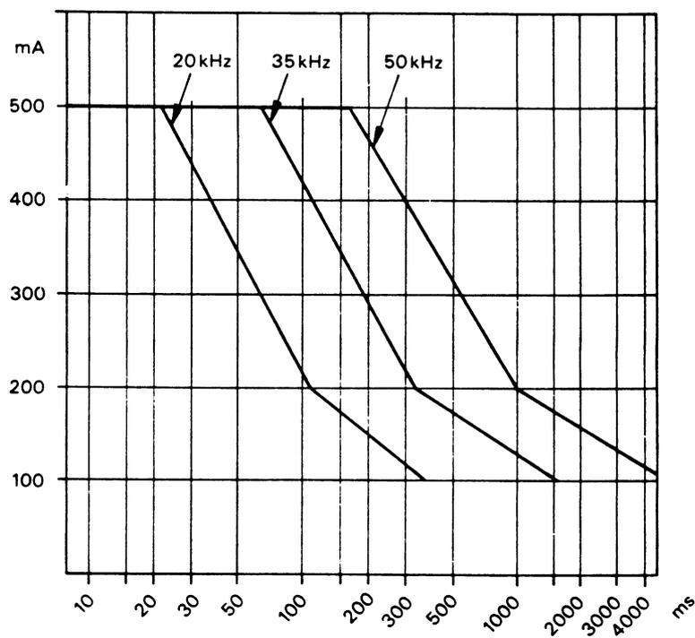
**Figure 23 — Limits for capacitive leakage current of HF-operated tubular fluorescent lamps**
