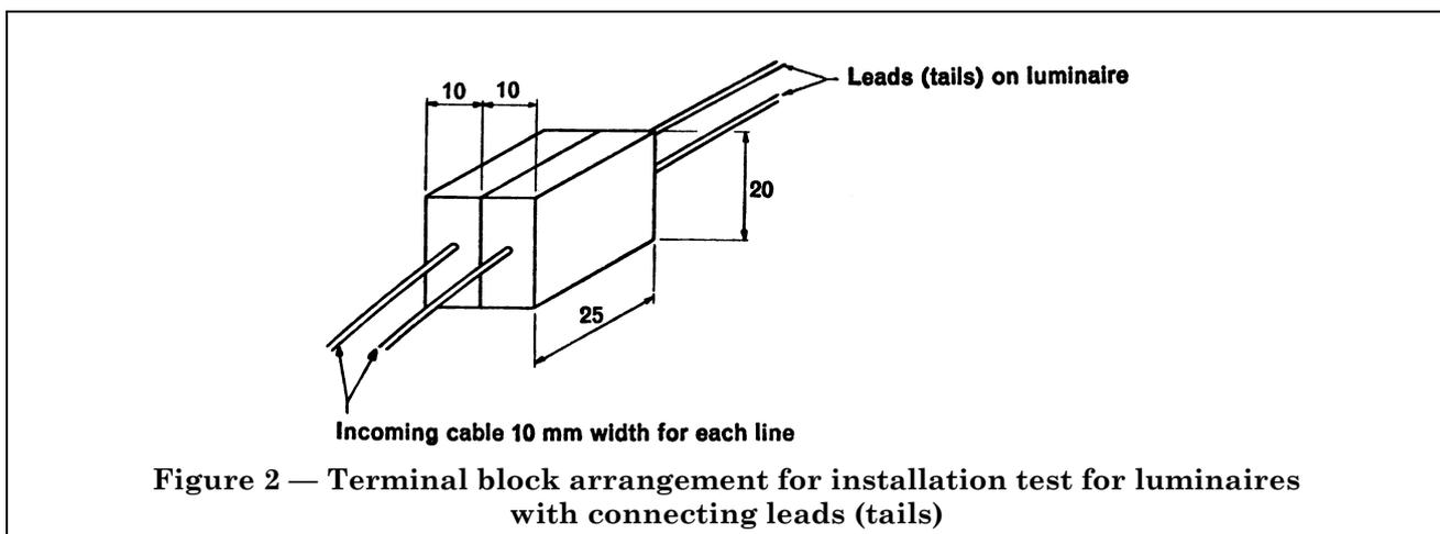
Figure 2 — Terminal block arrangement for installation test for luminaires with connecting leads (tails)
